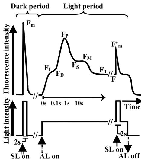
**Figure1.** Schematic diagram of the consecutive measurement of CFI method and saturation pulse method. All experiments were performed on attached cucumber leaves.
