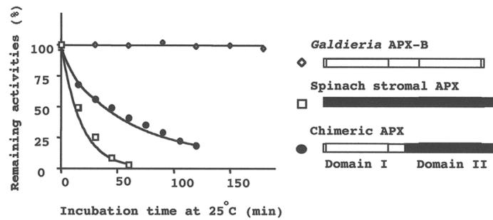
**Fig. 1 Change in activity of recombinant APXs after incubation under ascorbate-depleted condition.** (Left) Highly purified APX-B (diamond) and partially purified stromal APX (square) of spinach and chimeric APX (circle) were analyzed. After indicated times of incubation in 50 mM MES-KOH, 0.01 mM ascorbate and 0.1 mg/ml BSA (pH 7.0) at 25°C, enzymes were mixed with 0.5 mM of ascorbate and the activities were measured. (Right) Illustration of recombinant APX proteins used in this experiment.
