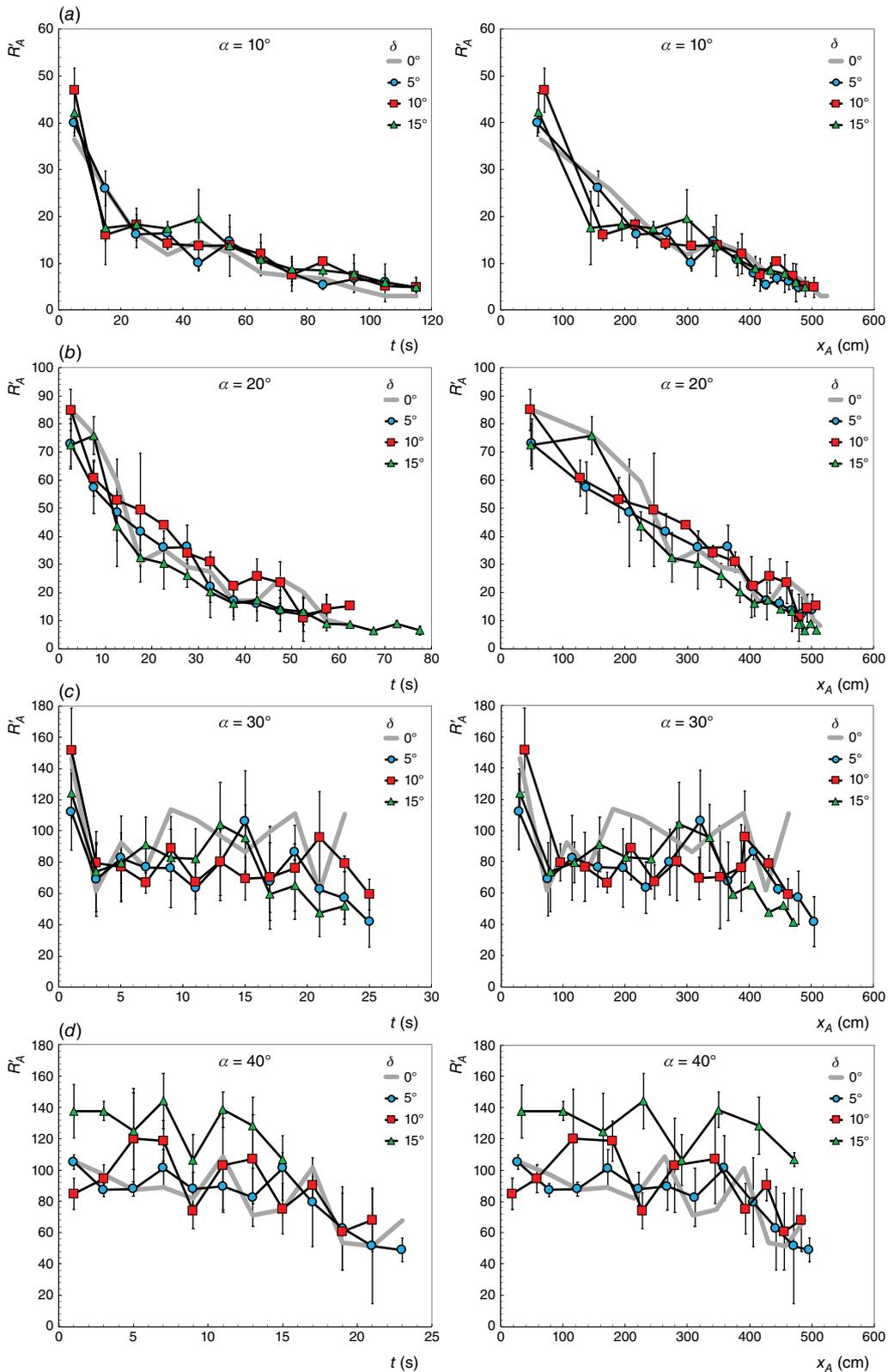
**Fig. 3.** Evolution of the non-dimensional ROS ( $R'_A$ ) as a function of the time and distance for different slope angles (a) and different rotation ( $\delta$ ) of the fire fronts. The average  $R'_A$  values of the three replications with 95% confidence intervals ( $\delta = 5^\circ, 10^\circ$  and  $15^\circ$ ) were plotted with the symmetrical boundary conditions ( $\delta = 0^\circ$ ): (a)  $a = 10^\circ$ , (b)  $a = 20^\circ$ , (c)  $a = 30^\circ$  and (d)  $a = 40^\circ$ .
