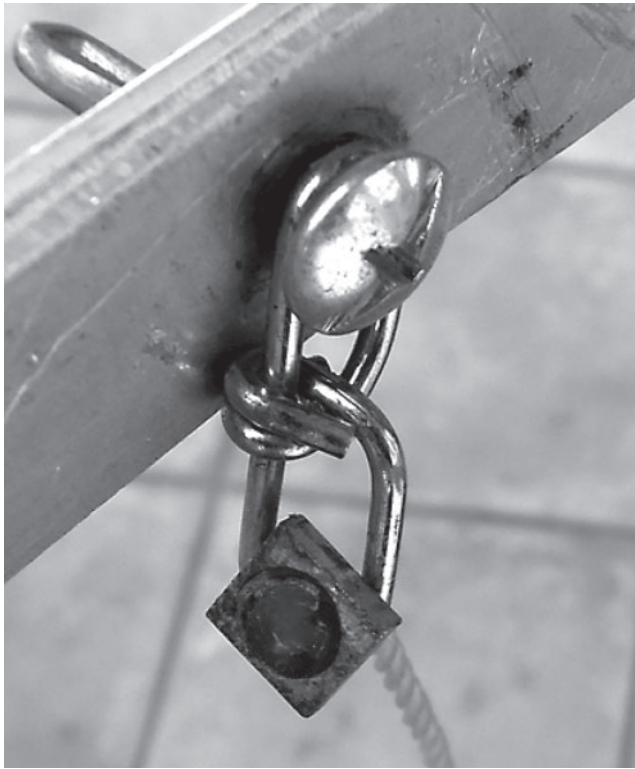
Fig. 3. A two-link piece of chain (see Table 2) acting as cord guide, which is part of trip-plate section of the trigger system: one link is fastened by a 6-mm × 18-mm gutter bolt (four of which are used as fasteners when erecting a trap in working configuration) and matching wing nut on the port side of the upper bar that is also used to secure the trap in a working configuration. Note that the second link serves as both a guide and stopper for ease of retrieval when setting a trap.
