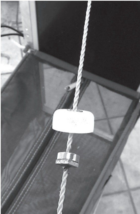
Fig. 5. Neodymium magnet with protective shield (see text) withdrawn for illustrative purposes connected to an 11-mm 2 metallic nut (Fig. 3). The cord is polyethylene, which is threaded through the openings of both connectors. To secure: heat is applied to melt the cord, which, being malleable, can be flattened, coated with an adhesive, and made flush on both mating surfaces.
