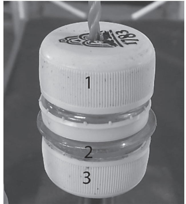
Fig. 6. A simple and effective magnet protector for use during storage using recycled materials: (1) and (3) plastic caps from a 1.25-L fruit juice bottle; (2) neck portion of bottle. To construct: the neck is severed, heated and, while in a melted hot phase, the bottom cap (3) is fused to the neck on cooling. For storage in pocket (Fig. 1b) the top cap with magnet is screwed back on the top of the neck, and, on folding the trap, the protector is stored in the side pouch (see text describing the need for protection during use and storage).
