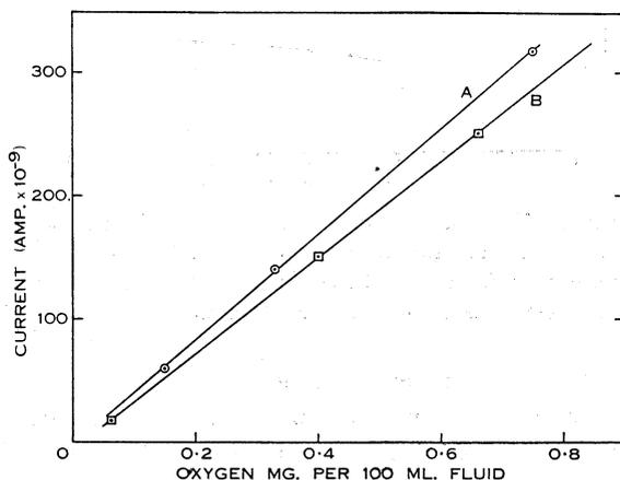
Fig. 3.—Current-oxygen tension curves of open electrode No. 2. Calibration was carried out using 0.15M NaCl at 37°C. containing known amounts of oxygen. Electrode potential 0.8 volt v. 0.15M calomel half-cell. Readings were taken 40 sec. after closing the switch.
