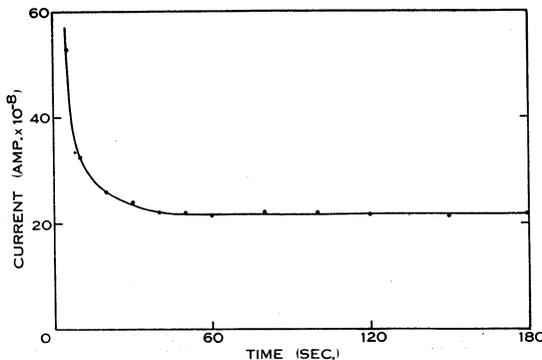
Fig. 2.—Time-current relationships of open electrode No. 2 in air-saturated 0.15M NaCl at 24°C. Electrode potential 0.8 volt *v.* 0.15M calomel half-cell.
