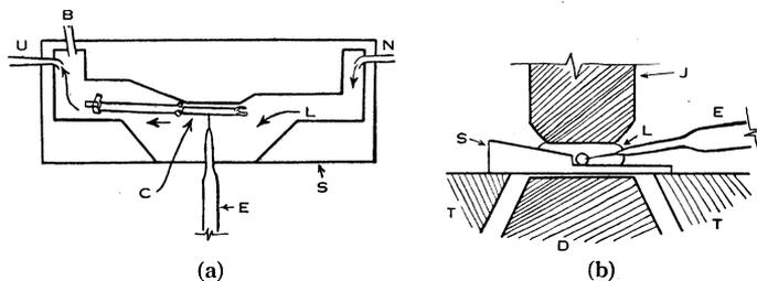
Fig. 1.—(Not to scale). (a) Plan of experimental arrangement. (b) Section. C, *Nitella* cell; E, microelectrode; S, "Perspex" slide; L, bathing solution; N, inflow of fresh solution; U, outflow of solution; B, agar salt bridge; J, microscope objective; T, microscope stage; D, microscope condenser.
