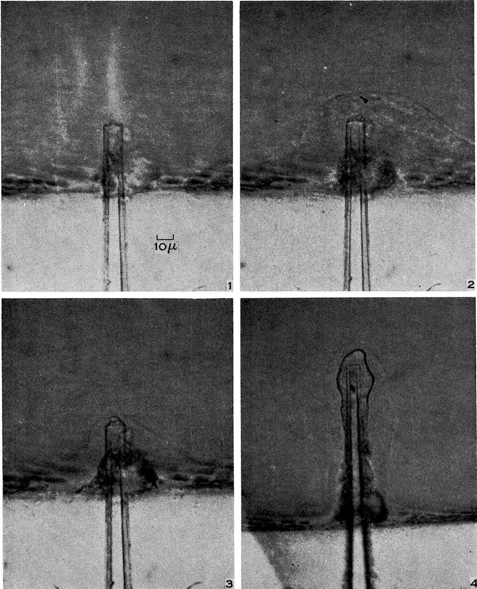
Photomicrographs of a microelectrode tip inserted into a *Nitella* cell. This tip is  $10\ \mu$  in diameter, i.e. rather larger than those generally used. Magnification  $\times c. 500$ .
