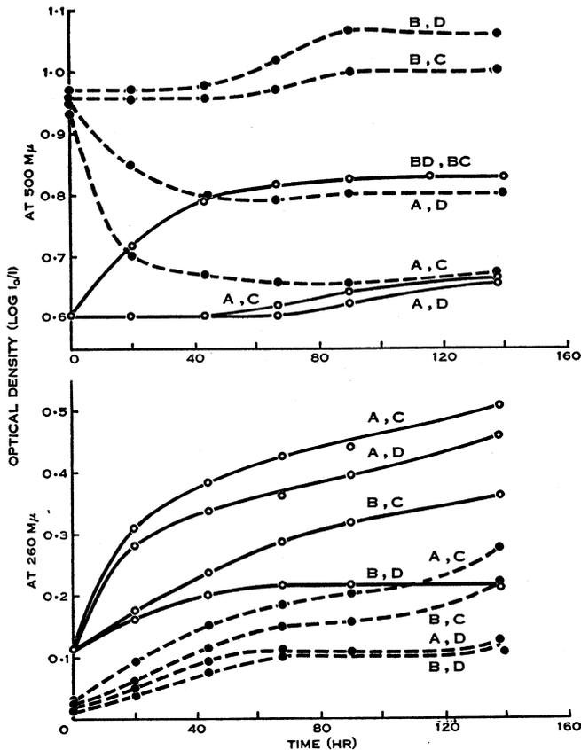
Fig. 1.—Storage of *M. lysodeikticus* (broken lines) and protoplasts at a concentration of 1 mg dry wt./ml in 1M sucrose. Optical densities at 500  $\mu$  measured on suspensions and at 260  $\mu$  on centrifuged supernatants. Conditions of storage indicated on curves: A, pH 6.5; B, pH 5.5; C, 15°C; D, 0°C.
