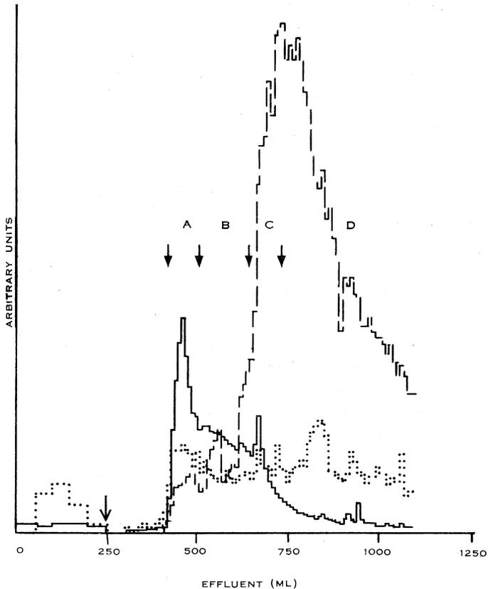
Fig. 9.—Sodium chloride gradient elution chromatography of a batch of *S. atra*  $\beta$ -glucosidase with a higher carbohydrate content and a very low enzyme activity. DEAE-cellulose, small column, standard conditions, 0.02M sodium acetate buffer at pH 4.1. ——— Enzyme; ..... protein; — — — carbohydrate. The arrows indicate the limits of the various fractions into which the eluate was divided.
