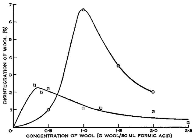
Fig. 1.—Disintegration of wool as a function of the amount of wool in 50 ml 98% formic acid when treated for 30 min at maximum power in the 300-ml round-bottomed Pyrex vessel with the 9 : 1 probe 0.5 cm above the bottom (○), or with the 4 : 1 probe 0.5 cm below the surface of the liquid (□).
