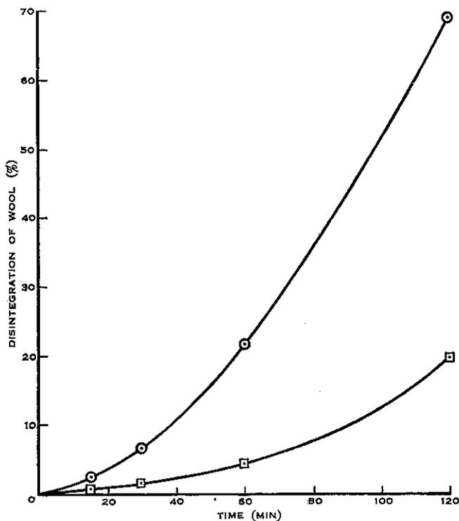
Fig. 2.—Disintegration of wool as a function of time of treatment in 50 ml 98% formic acid at maximum power in the 300-ml round-bottomed Pyrex vessel with the 9 : 1 probe 0.5 cm above the bottom of the vessel ( $\circ$ ), or with the 4 : 1 probe 0.5 cm below the surface of the liquid ( $\square$ ).
