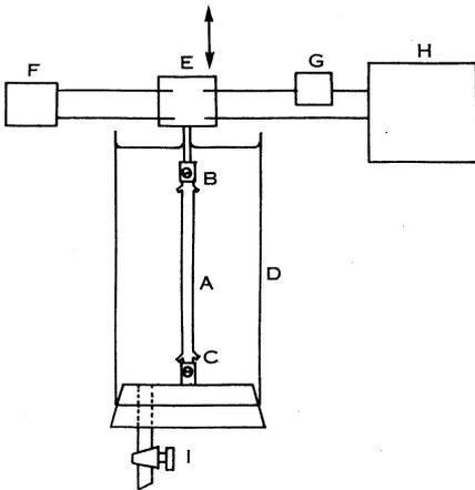
Fig. 1.—Schematic diagram of experimental apparatus. Plant cell *A*, in container *D*, is clamped between *B* and *C*. End *B* is attached to transducer *E* which is vertically adjustable. Excitation voltage is provided by *F*, a 9 V battery. Potentiometer *G* provides a biasing voltage for the transducer output which is displayed on recorder *H*. The bathing solution may be drained at *I*.
