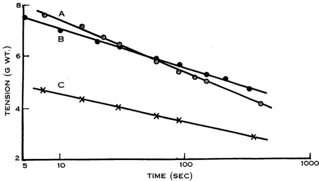
Fig. 2.—Typical stress relaxation of internodal cells and cell wall strips. *A*, internodal cell of length approximately 70 mm, extended 0.18 mm. *B*, same cell as in *A*, but extended a further 0.23 mm. *C*, longitudinal cell wall strip of length 50 mm extended 0.13 mm.
