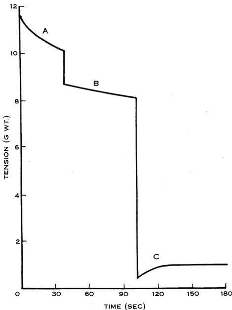
Fig. 3.—Cell wall response to extension and partial and total return to original length. *A*, stress relaxation after sudden extension. *B*, the continuation of relaxation of residual tension after partial release of extension. *C*, increase in tension after almost total return to original length.
