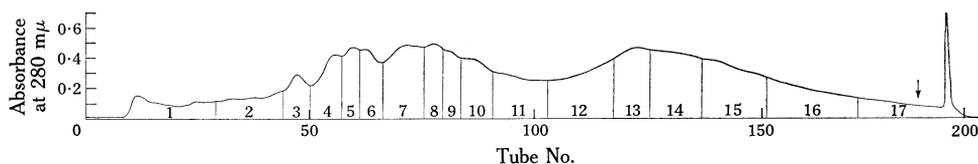
Fig. 1.—Chromatographic separation of 1 g of high-sulphur proteins into 17 fractions on DEAE-cellulose at pH 4.5. Experimental conditions are given in the text. The arrow indicates change to eluent with ionic strength 1.0. Yields of fractions (mg): 1, 24; 2, 35; 3, 38; 4, 48; 5, 35; 6, 46; 7, 71; 8, 32; 9, 29; 10, 43; 11, 57; 12, 78; 13, 62; 14, 88; 15, 88; 16, 76; 17, 48. Total recovery, 0.90 g.
