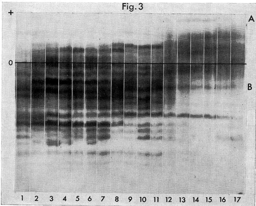
Figs. 2 and 3.—Electrophoretograms run at pH 6.5 (Fig. 2) and 3.5 (Fig. 3) showing comparative peptide maps of tryptic (Fig. 2) and chymotryptic (Fig. 3) digests of the 17 high-sulphur protein fractions defined in Figure 1. O, origin.
