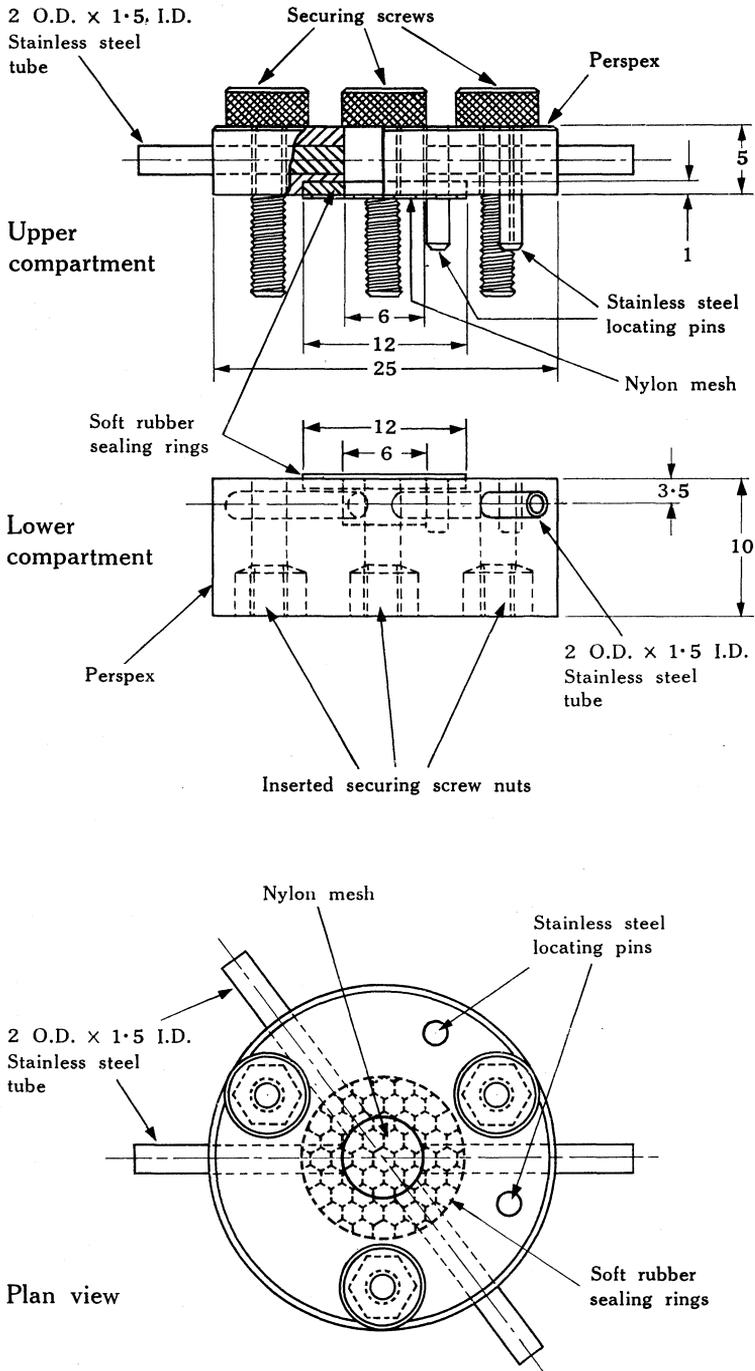
Fig. 1.—Construction details of the solution-flow porometer. All measurements given in millimetres.
