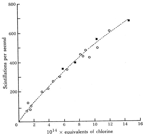
Fig. 1.—Calibration curve for chlorine obtained by spot analysis of small, flat, rectangular crystals of KCl (○) and NaCl (■). A beam current of approximately 1.2 nA was used at an accelerating voltage of 20 keV. Crystal sizes were measured by scanning electron microscopy.
