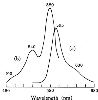
Fig. 3. The pronase-, heat-treated desulfovirdin, in 0.1 M phosphate buffer (pH 7.0), was used in these experiments. (a) Fluorescence emission spectrum when excited at 385 nm. (b) Excitation spectrum obtained by recording the fluorescence at an emission wavelength of 630 nm.
