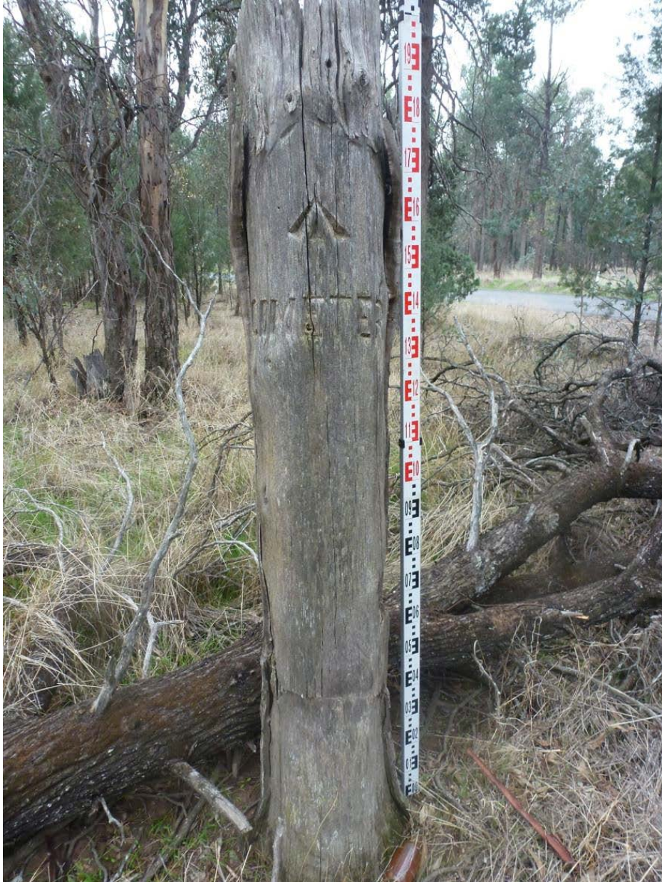
Fig. S3. A dead Callitris glaucophylla post, surveyed in 1910, used to mark out a planned cemetery portion in State Forest Reserve. Photograph: P. Spooner.
