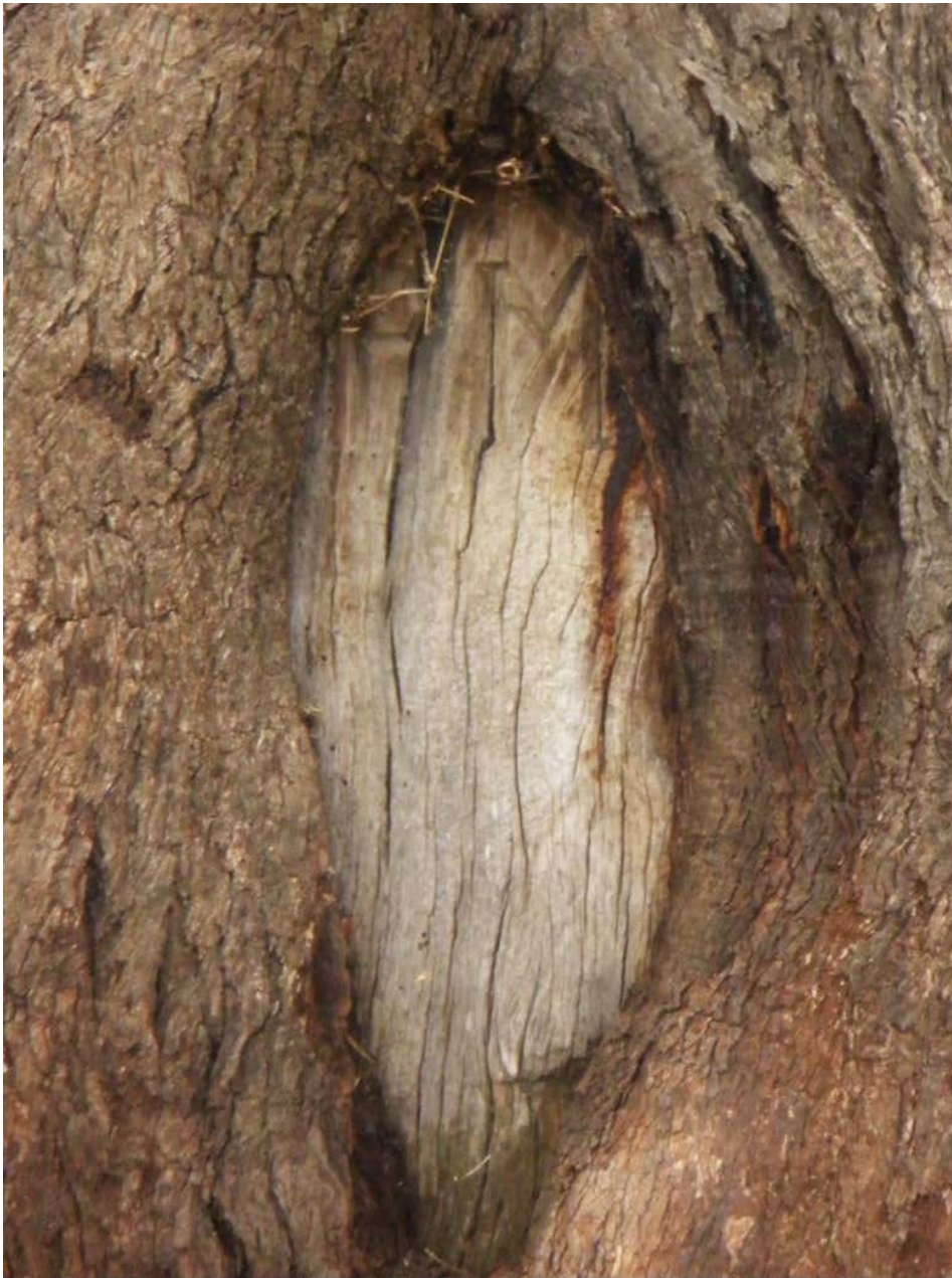
Fig. S2. Example of permanent marker (PM) reference tree ( Eucalyptus melliodora ) surveyed in 1962. The 'PM' marking which is chiselled is in excellent condition (top of blaze face), but is becoming hidden by blaze overgrowth. Photograph: B. Thompson.
