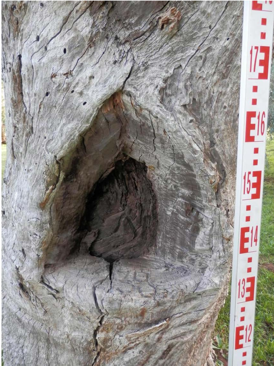
Fig. S4. Example of a blaze ‘chop-out’, where a surveyor in recent times has chopped out the overgrowth of a large box tree (probably Eucalyptus melliodora ), to reveal the original blaze. This tree was first surveyed in 1936, where the portion number ‘238’ has been re-chiselled on the lower lip of the chop-out. Located in the Holbrook focus area. Photo: P. Spooner.
