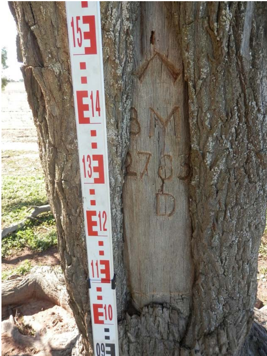
Fig. S1. Example of a benchmark (BM) survey reference tree ( Callitris glaucophylla ), showing an (abbreviated) broad arrow (normally shown as ‘↑’), a ‘BM’ partly obscured, the number ‘2783’ indicating its position on a survey traverse, and the initial ‘D’, for surveyor Mr J. D. Dalglish, who blazed this tree in 1932 (NSW WIC 1932). The marker ruler shows the height of blaze features above ground level at the base of the tree. Photograph: P. Spooner.
