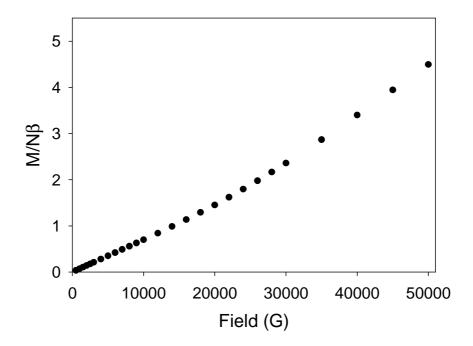
**Fig. S4.** Field dependence of the magnetization at 2 K for **1**.
