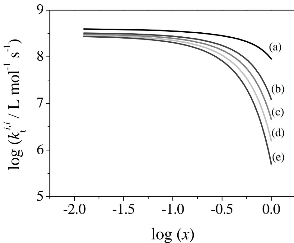
**Figure 4.** log-log plot of the chain length and conversion dependent termination rate coefficient,  $k_t^{i,i}(x)$ , vs conversion,  $x$ , extracted from the 3-dimensional  $\log k_t^{i,i}(x)$  vs  $\log i$  vs  $x$  surface profile for the RAFT-mediated polymerization of styrene (STY, 8.15 M) using the 6-arm star RAFT agent dipentaerythritol hexakis(3-(s-benzyltrithiocarbonyl)propionate) (6-BTTC) with 1,1- azobis (cyclohexanecarbonitrile) (VAZO88) as initiator at 90 °C
