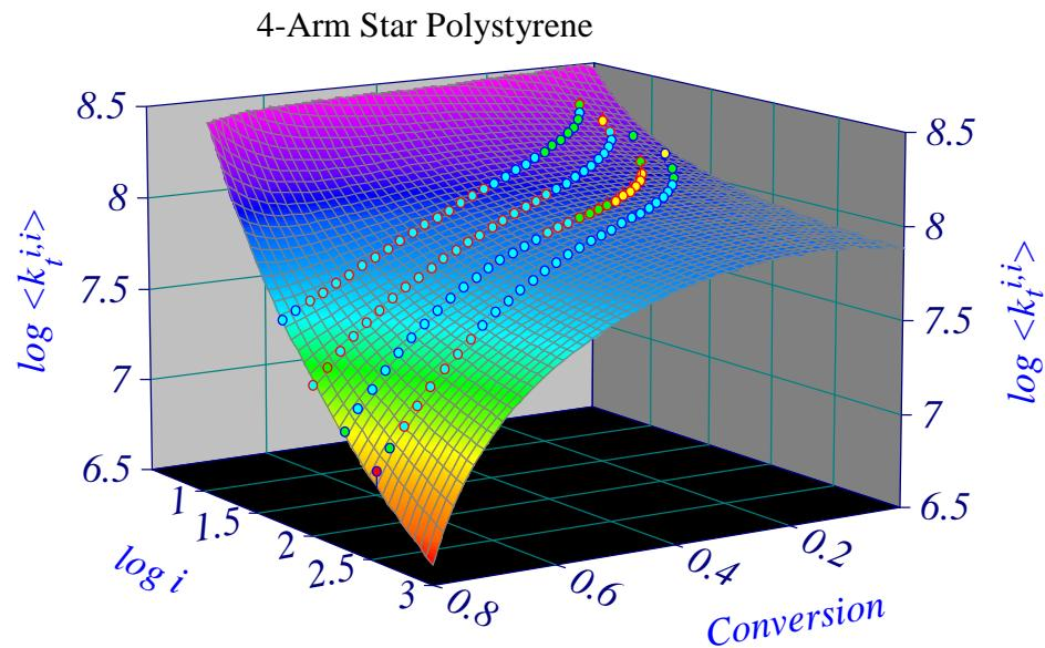
**Figure S1.** Three dimensional plot of the termination rate coefficients,  $k_t$ 's, for RAFT-mediated styrene (STY) polymerized in bulk and in the presence of the 4-arm star RAFT agent *pentaerythritoltetrakis(3-(s-benzyltrithiocarbonyl)propionate)* (4-BTTC), initiated with 1,1- azobis (cyclohexanecarbonitrile) (VAZO88) at 90 °C. The data was fit with a surface plot using TableCurve 3D software ( $r^2 > 0.99$ ). Drop lines indicate some minor deviation from the surface fit function.
