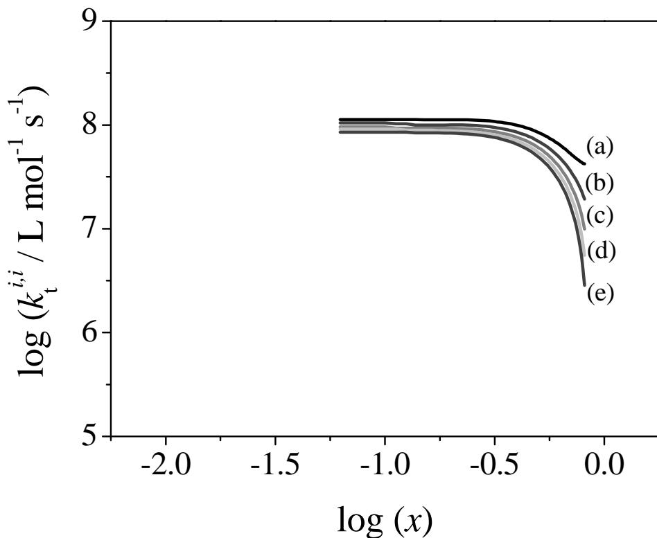
**Figure 3.** log-log plot of the chain length and conversion dependent termination rate coefficient,  $k_t^{i,i}(x)$ , vs conversion,  $x$ , extracted from the 3-dimensional  $\log k_t^{i,i}(x)$  vs  $\log i$  vs  $x$  surface profile for the RAFT-mediated polymerization of styrene (STY, 8.15 M) at 90°C using 4-arm star RAFT agent pentaerythritoltetrakis(3-(s-benzyltrithiocarbonyl)propionate) (4-BTTC), initiated with 1,1-azobis(cyclohexanecarbonitrile) (VAZO88) at 90 °C.
