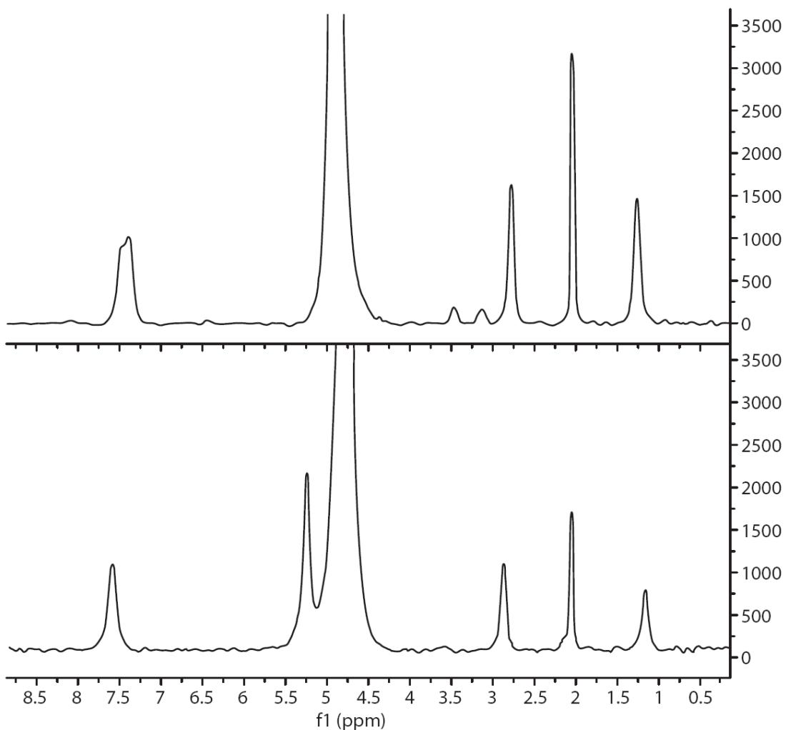
**Figure S-1. Top;** a representative  $^2\text{H}$  NMR spectrum of methamphetamine/HCl in water. The peaks in the spectrum from low field to high field can be assigned as; phenyl, water, methine, benzyl, *N*-methyl, acetonitrile, methyl.
