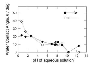
**Figure 1.** Plot showing the measured contact angle using water droplets at two CP films, each generated from electrolysis of  $0.42 \text{ mM CBD} + 0.1 \text{ M H}_2\text{SO}_4$  at 600 s. Each film was sonicated in pH buffered solutions sequentially from either low to high pH or the reverse. Closed and open circles indicate the direction of sampling.
