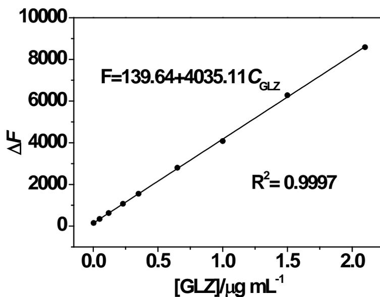
Fig S1 The standard calibration graph of GLZ.
