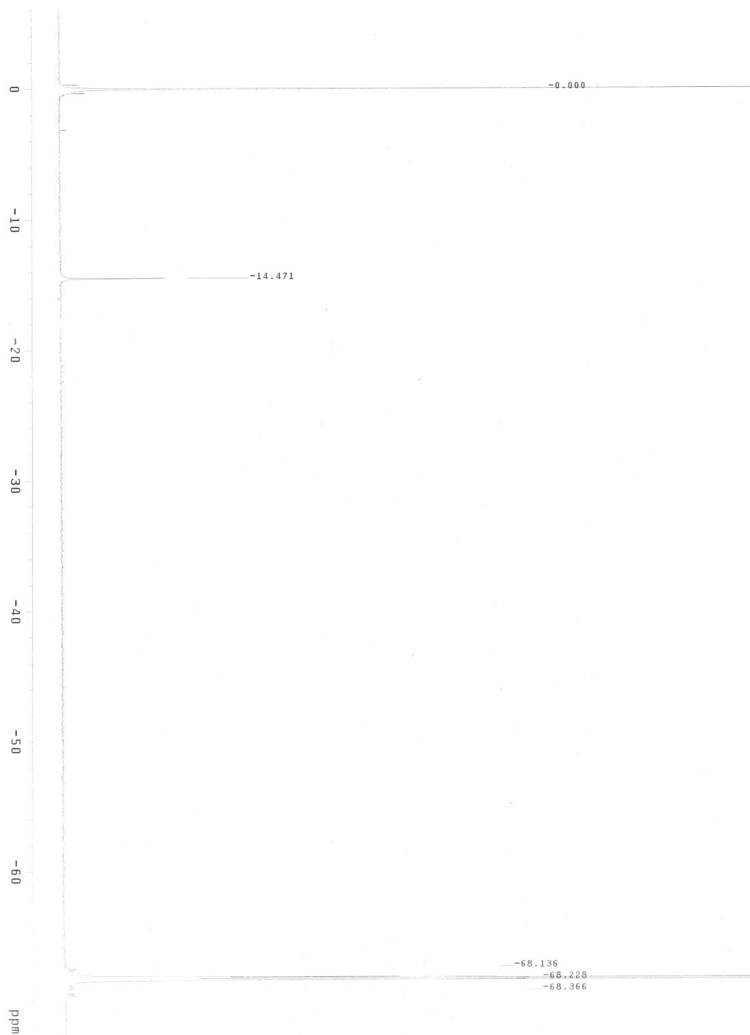
Figure S12. ^{29}\text{Si} NMR ( \text{CDCl}_3 ) spectrum of (p\text{-HSiMe}_2(\text{CH}_2)_2\text{C}_6\text{H}_4)(c\text{-C}_6\text{H}_{11})_7\text{Si}_8\text{O}_{12} ( 5 )
