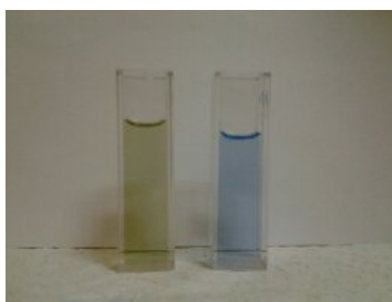
Figure S13. The change of the absorption of dye 7j after one day is seen even with naked eye (green –in MeOH; blue - in EtOH).
