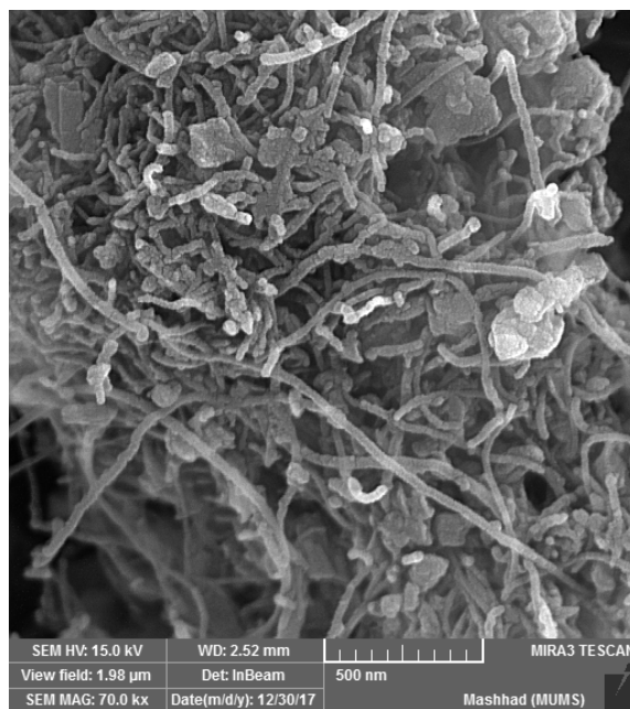
Fig. S4. The FE-SEM image of FMMWCNTs@CPA@SMTU@Pd II NPs ( IV ).
