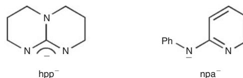
**Fig. 6.** Ligands (L<sup>−</sup>) employed in the formation of [L<sub>6</sub>Li<sub>8</sub>H][A] complexes (npaH = 2-*N*-pyridylaniline).
