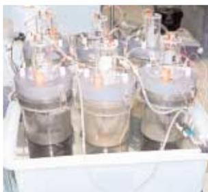
Core samples from Lake Carramar, Australia, were used in laboratory bioreactors (see Figure) to test three forms of calcite as active barriers to prevent phosphorus release from sediments (linked to algal blooms). The two precipitated calcite products (possessing the greatest surface area) proved most effective: a 2% layer of SoCal reduced phosphorous release by 100 times that of the control; ESCal, a cheaper Australian product, may go to further trials.
