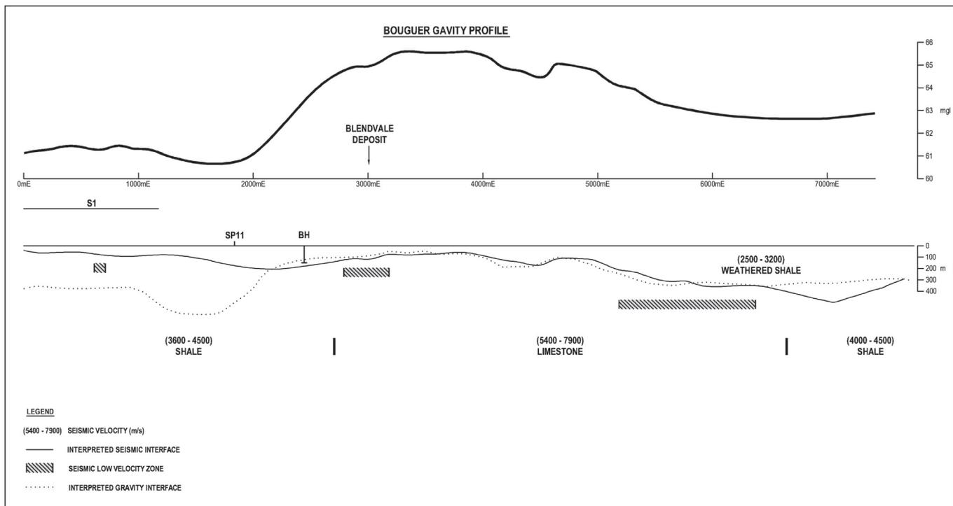
Fig. 1. Early gravity and seismic refraction interpretations over the Blendvale, MVT deposit.
