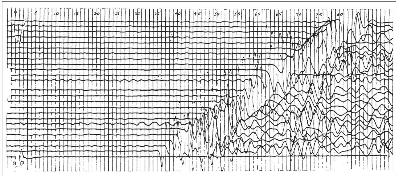
Fig. 2. Long-offset analogue seismic refraction record from SP11 over the western margin shales/siltstones.
