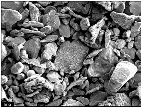
Fig. S2 SEM micrographs of MZVI (a) before using in soil washing and (b) recovered from the soil washing process.
