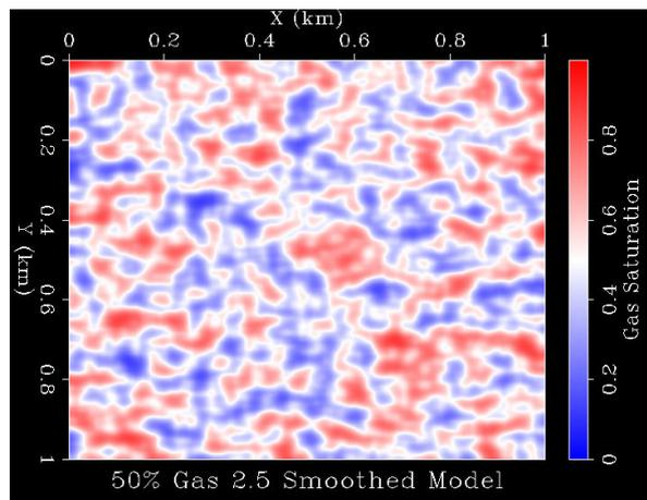
**Figure 4. A smoothed version of 50% gas saturation map with the smoothing range significantly larger than the patch size.**
