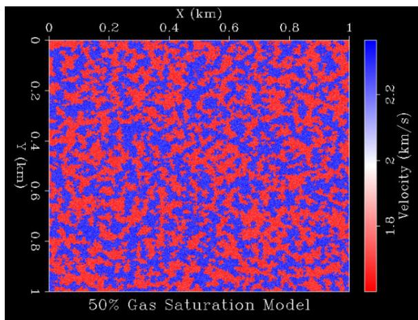
**Figure 1. One of the velocity models used in the initial modelling. This model represents a cross-section of a reservoir rock 50% gas saturated and 50% water saturated.**
