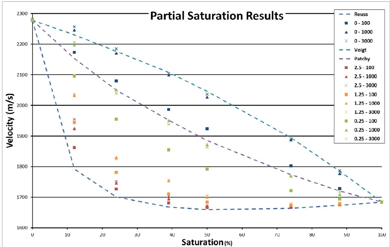
Figure 2. The velocities measured in this study. The first number for each series in the legend describes the amount of smoothing that was applied to the velocity model; the second number is the central frequency of the input plane wave. The dashed lines are the three theoretical bounds.
