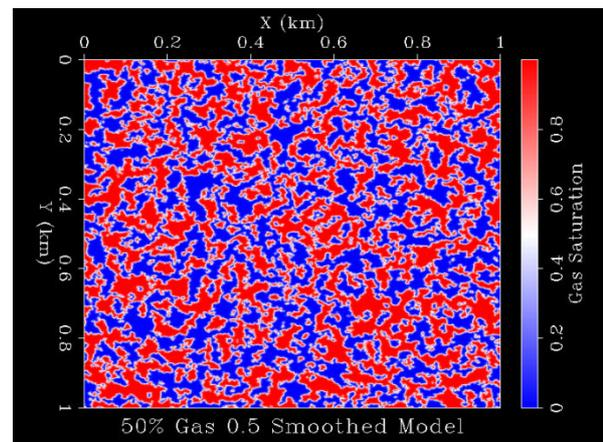
**Figure 3. A smoothed version of 50% gas saturation map with the smoothing range smaller than the patch size.**
