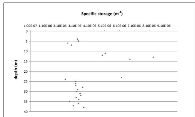
**Figure 2: specific storage values determined through cross-hole seismic survey.**
