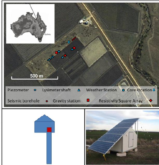
**Figure 1: (top) Instrumentation at the field site in the Liverpool Plains; (bottom left) schematic of the foundation for the gravimeter; (bottom right) the solar powered gravity station in the field.**
