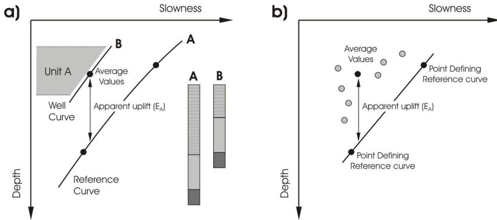
**Figure 2. Idealised evolution of seismic slowness during maximum burial (A), subsequent exhumation (B). Apparent exhumation ( $E_A$ ) is estimated from the displacement, along the depth axis of the sonic slowness/depth relationship of the exhumed sequence (B) from that of the normally compacted or reference, sequence (A). Modified from Hillis (1993).**
