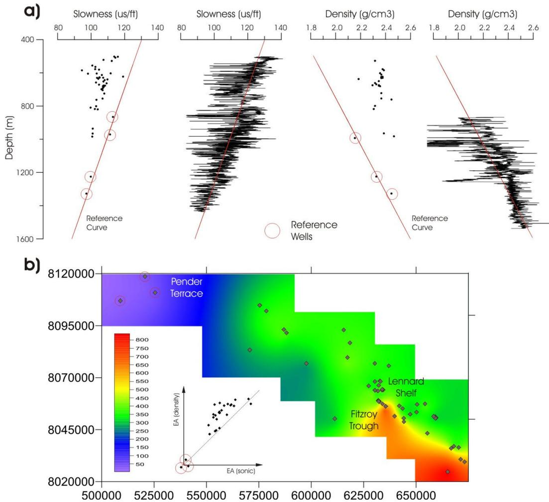
**Figure 3. Estimation of tectonic uplift of the Noonkanbah Formation based on sonic and bulk density logs. See Figure 1 for location of map.**
