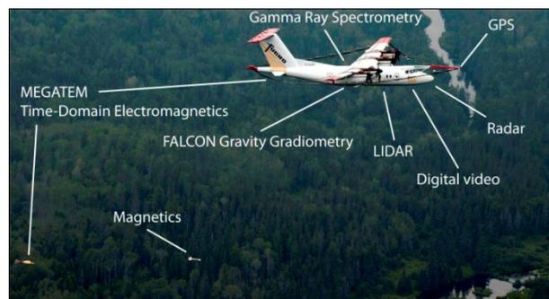
**Figure 1.** Multi-sensor airborne platform operated by Fugro Airborne Surveys.
