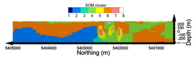
**Figure 8.** Vertical cross-section along line L50 of pseudo-lithological domains obtained from self-organized map of 3D conductivity, magnetic susceptibility and density models.
