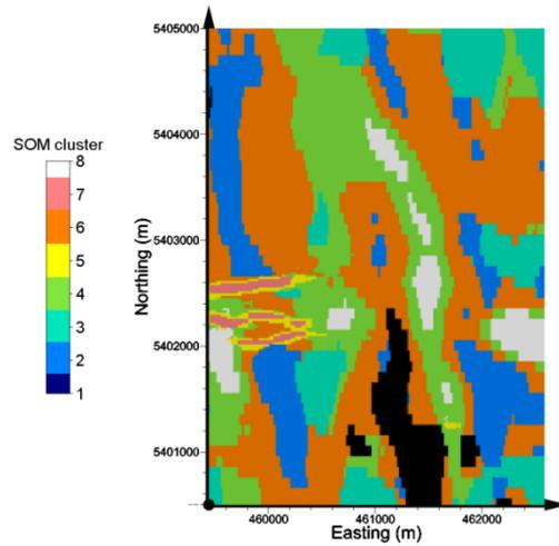
**Figure 7.** Horizontal cross-section of pseudo-lithological domains obtained from self-organized map of 3D conductivity, magnetic susceptibility and density models.
