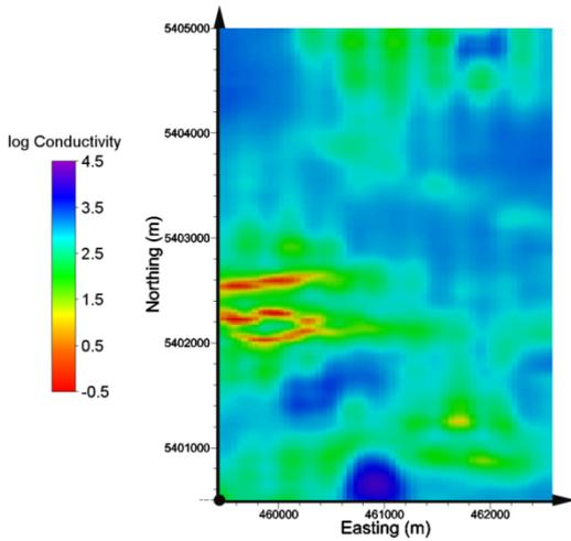
**Figure 4.** Horizontal cross-section of conductivity obtained from 3D inversion of MEGATEM II dB/dt data. The sub-vertical bedrock conductors beneath line L50 can clearly be seen.
