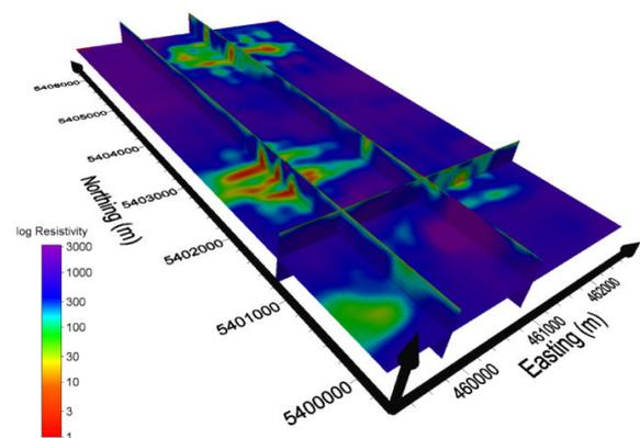
**Figure 3.** Perspective of the 3D resistivity model obtained from 3D inversion of MEGATEM II dB/dt data. Sub-vertical bedrock conductors beneath line L50 can clearly be seen.
