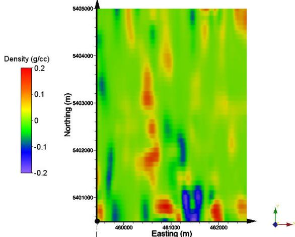
**Figure 6.** Horizontal cross-section of density contrast obtained from 3D inversion of multiple tensor component FALCON gravity data.
