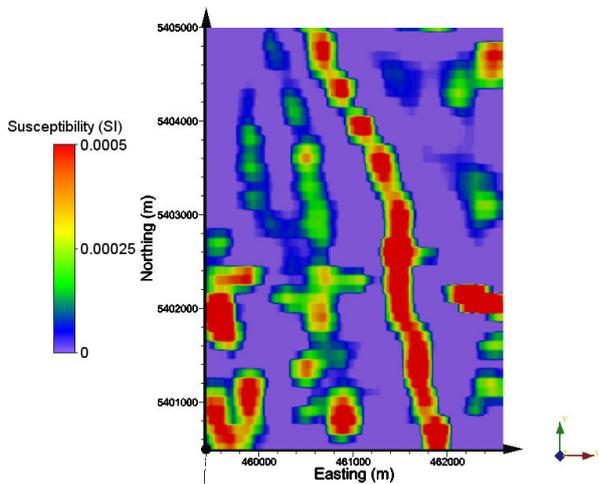
**Figure 5.** Horizontal cross-section of magnetic susceptibility obtained from 3D inversion of total magnetic intensity (TMI) data. The diabase dykes are clearly seen in these results.
