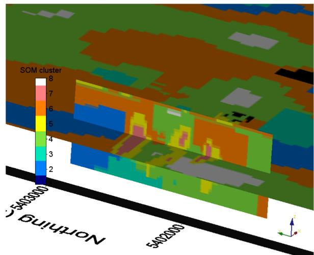
**Figure 9.** 3D perspective view of the pseudo-lithological domains obtained from self-organized map of 3D conductivity, magnetic susceptibility and density models. Vertical cross section for line L50 is shown.
