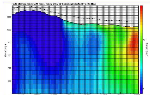
**Figure 1. Illustration of model mesh for 2D inversion. Since the algorithm takes into account the topography and ZTEM bird terrain clearance along each line, air cells are an integral part of the finite-element model.**
