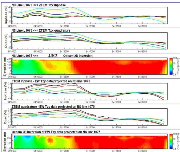
**Figure 7. Forrestania ZTEM profiles across sulphide IR2, indicated by arrow, with corresponding inversion results. A portion of Tzx profiles of north-south line 1075 are shown in the top panels; the profiles derived from the Tzy data of the east-west lines are shown in the bottom panels.**
