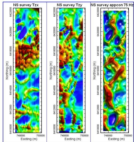
**Figure 8: North-south survey data. Conductivity structure at an elevation of 120 m ASL, derived from 2D inversion of Tzx (left) and Tzy (center) data, and 75 Hz apparent conductivity (right).**
