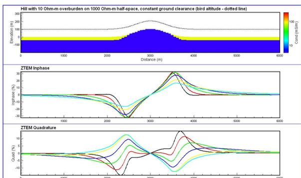
Figure 3. The ZTEM response of a resistive hill (1000 Ohm-m) flanked by conductive overburden (10 Ohm-m) for a receiver terrain clearance of 100 m.
