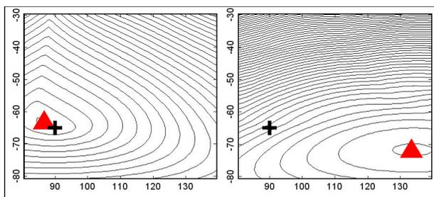
**Figure 3. Declination-inclination plots for (left) Maxi-min and (right) RTP cross-correlation methods for high-inclination (-65°) dipole magnetization (cross – actual direction, triangle estimated)**
