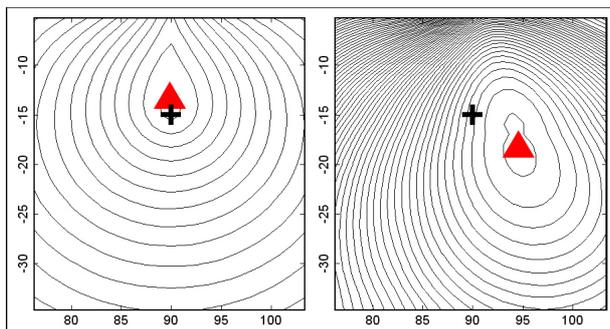
**Figure 2. Declination-inclination plots for (left) Maxi-min and (right) RTP cross-correlation methods for low-inclination (-15°) dipole magnetization (cross – actual direction, triangle estimated)**
