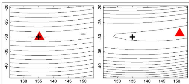
Figure 6. Declination-inclination plots for (left) Maxi-min and (right) RTP cross-correlation for across-axis magnetization (cross – actual direction, triangle estimated)
