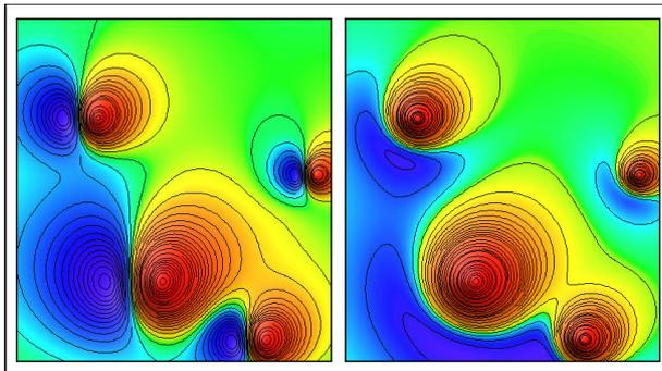
**Figure 7. TMI anomalies for magnetizations (inclination, declination): a)  $-15^\circ$   $90^\circ$  and b)  $-65^\circ$   $90^\circ$ . Geomagnetic field:  $0^\circ$   $-60^\circ$ .**
