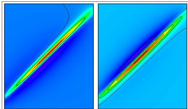
Figure 4. TMI anomalies for magnetizations (inclination, declination) a) parallel to axis: 45°, -30°, b) perpendicular to axis: 135°, -30°
