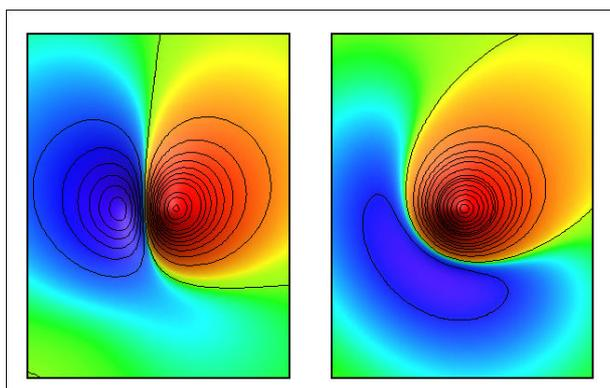
**Figure 1. TMI Anomalies for magnetizations (declination, inclination): a) 90° -15° and b) 90° -65° in a geomagnetic field Declination 0°, Inclination -60°**
