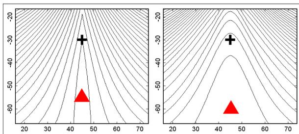
Figure 5. Declination-inclination plots for (left) Maxi-min and (right) RTP cross-correlation for along-axis magnetization (cross – actual direction, triangle estimated)
