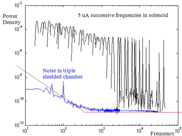
**Figure 2.** Early test of a prototype sensor to establish relationship between signal and noise. Each black peak corresponds to a power density equivalent to an amplitude of 1 pT per sqrt(Hz). The triple walled chamber shielding effectiveness decreases below 300 Hz.
