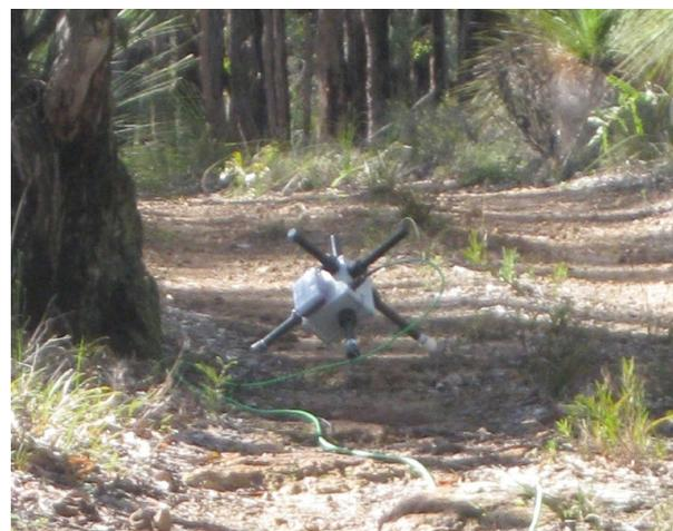
**Figure 5:** Three component ARMIT sensor in the field. The upper case contains accelerometer and orientation sensors so that measured data may be numerically rotated to the x, y, z or E, N, UP directions
