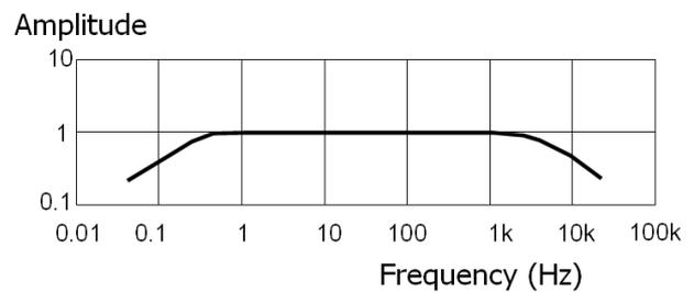
**Figure 4:** Amplitude sensitivity as a function of frequency to show 0.1 to 10 kHz bandwidth for the sensor
