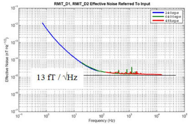
**Figure 3:** Noise level of ARMIT sensor measured in Utah. Due to DAS limitations, the noise at low frequencies (<10 Hz) is overestimated on this plot.
