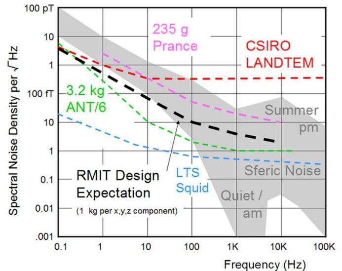
**Figure 1 Typical Sferic noise range (grey), and specifications of miniature Prance et al current sensor (magenta), CSIRO Landtem SQUID sensor (red), Zonge ANT/6 AMT sensor (green), and target ARMIT sensor (black). Fluxgate sensors have noise levels about 5 pT/ $\sqrt{\text{Hz}}$  and lie well above the sferic noise. LTS noise levels on this plot are lab levels, and underestimate those achieved in the field**
