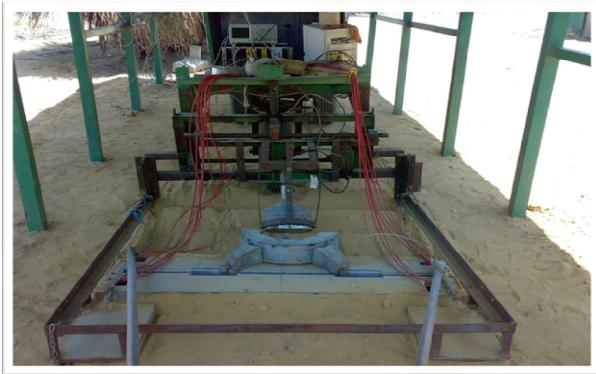
Figure 3. Photograph of Egyptian Scanning Landmine Detector, ESCALAD.
