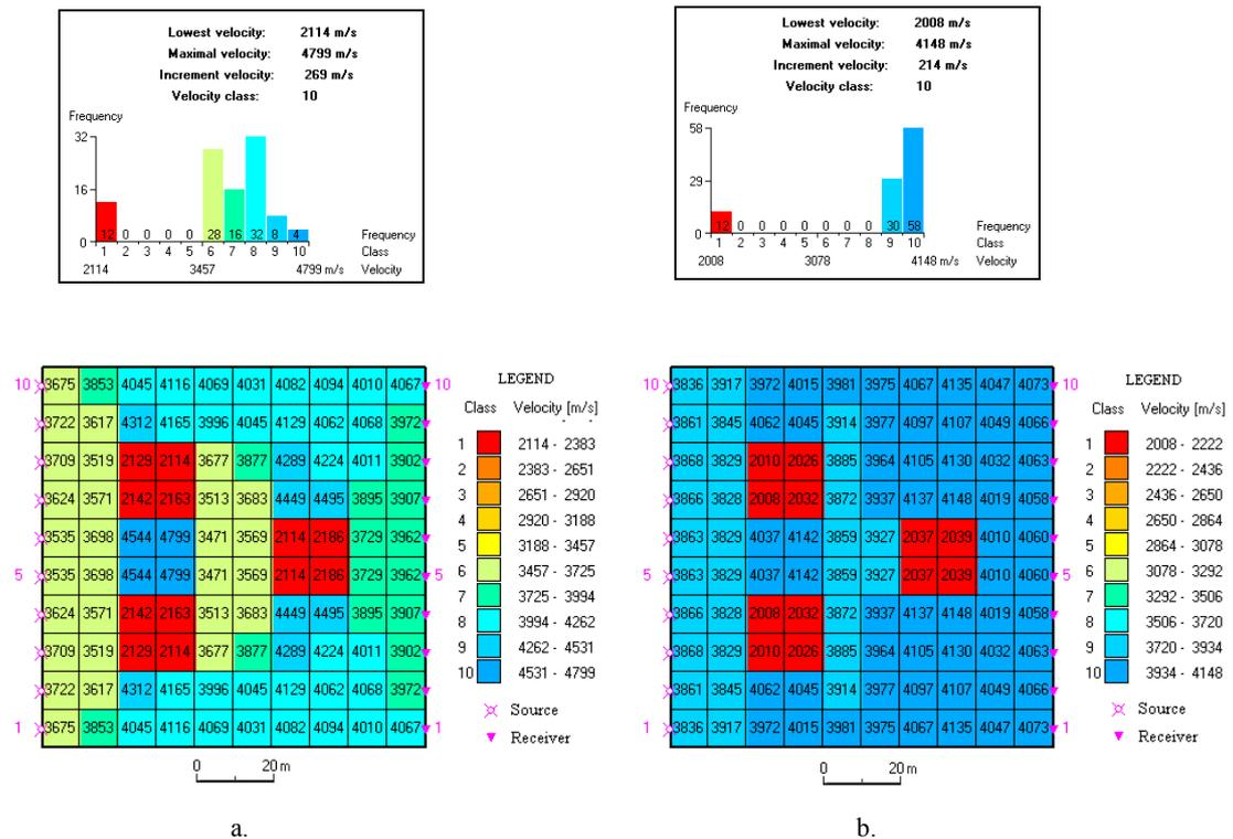
Figure 2. Tomography inversion for the model of a medium characterized by a high velocity (4000 m/s) containing three enclaves with low velocity (2000 m/s). This figure represents the results obtained by the matrix inversion method (a) and by our procedure (b) for a dataset acquired on an incomplete recording array (seismic sources and receivers on the two opposed sides of tested panel). On the upper row are depicted the velocity diagrams and on the down row the velocity maps are illustrated.
