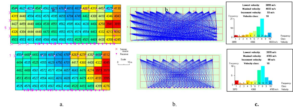
Figure 4. Velocity tomography results for a pillar situated at +240 m horizon of Praid halite mine (100 km N. Brasov, Romania). Comparative results for the same panel in case of a quasi-complete seismic array surrounding panel (upper row), respectively simulated incomplete field array (bottom row). The columns represent: a. the plan view of the velocity distributions; b. the raypath panel coverages; c. the histograms of velocity values.
