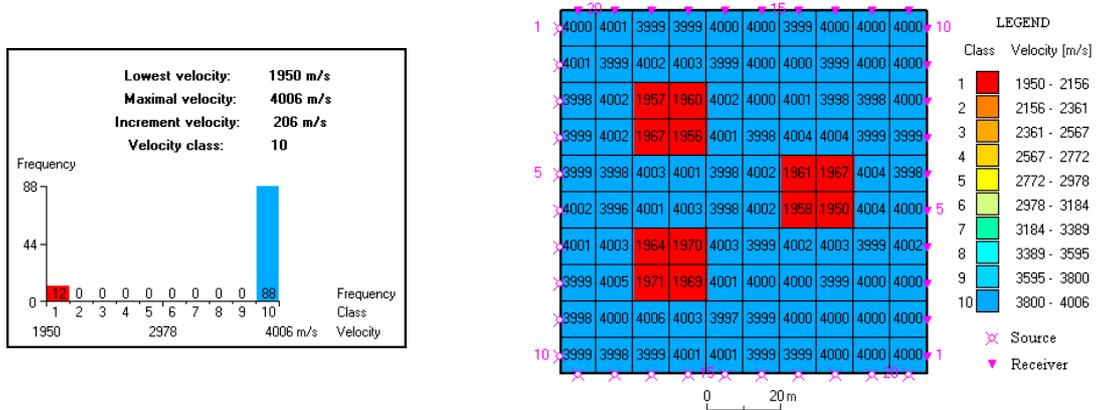
Figure 1. Tomography inversion for the model of a medium characterized by a high velocity (4000 m/s) containing three custom-defined enclaves with a low velocity (2000 m/s). This figure represents the results obtained by the matrix inversion method for a data set acquired on a recording array located completely around the panel: the histogram of velocity values (left) and the plan view of the velocity distribution (right).
