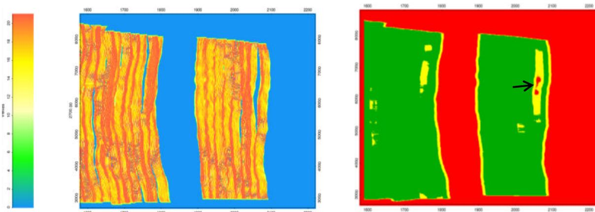
**Figure 3 Left: the fold achieved at the far offset interval. Right: the acceptability plot. The red area on the acceptability plot (arrowed) highlights where additional infill is needed to maintain image quality**
