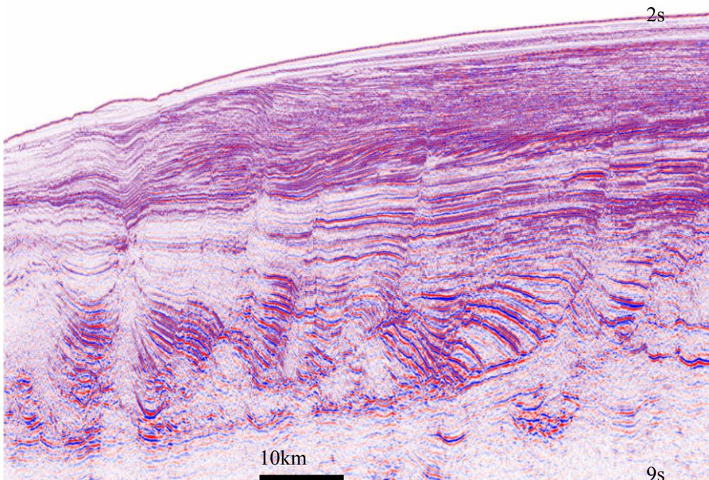
Figure 6 Seismic cross-line image after final Time Migration, down to 9 second twt with 30m cross-line bin size.
