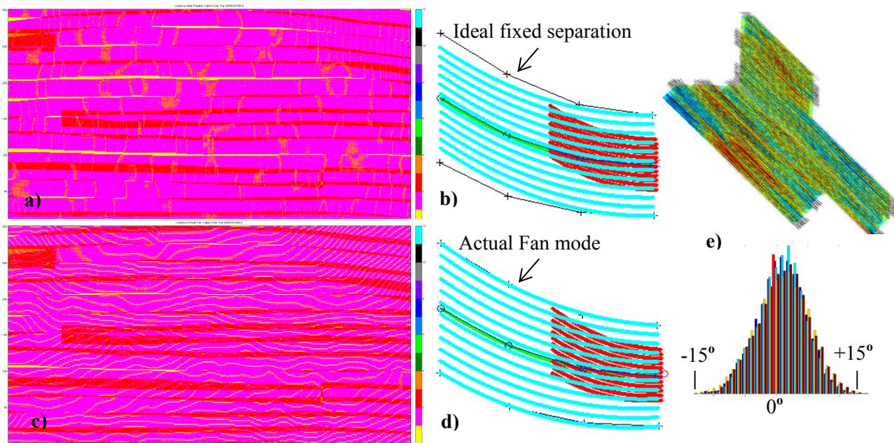
Figure 5 a) single offset fold (8km), yellow = empty cell, cables fixed separation as in b), cyan=receivers, red=midpoints, c) single offset fold (8km), yellow = empty cell, cables fixed separation as in d), same feather, same saillines, same channel count, e) Survey Feather map and histogram 780,000 shots.
