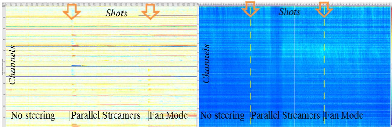
Figure 4 Single Sail-line: Left: streamer depth, Right: RMS noise plot. For each shot (x- axis), the depth or RMS noise is plotted in colour for each receiver (y- axis), arrows mark the shot where the steering mode was changed.
