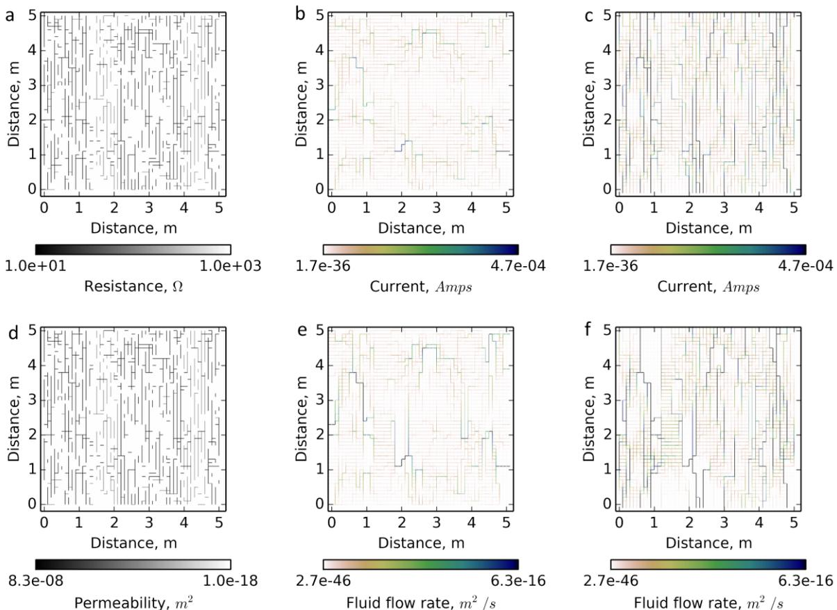
**Figure 2.** Two dimensional electrical random resistor network representing a  $5 \times 5$  m fractured rock mass with fault diameter 1 mm and fluid resistivity  $0.1 \Omega m$ . Probability of connection is 0.1 in the horizontal direction and 0.5 in the vertical
