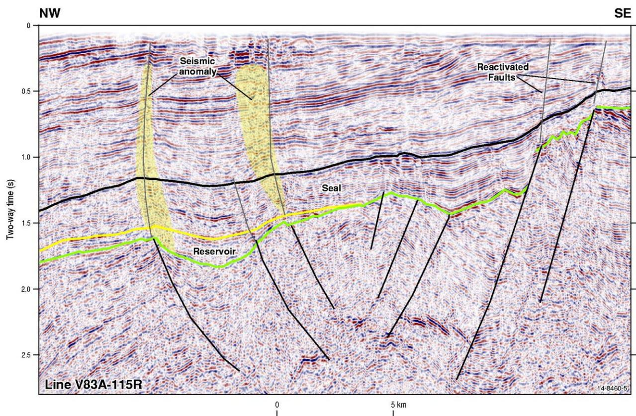
Figure 1. Sesimic line showing examples of reactivated faults and seismic anomalies in the southern Vlaming Sub-basin. The location of the line is shown in Figure 2.
