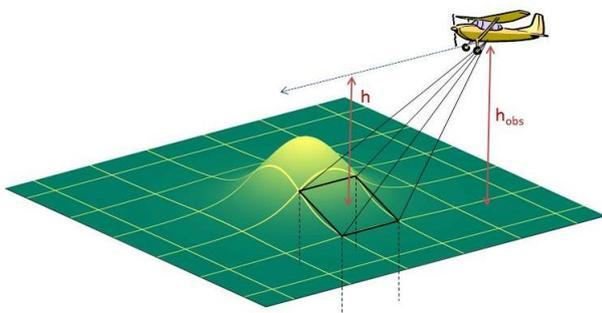
**Figure 2.** Schematic showing the parameterization of the topography using prism sources with slanted top surfaces relative to the detector.
