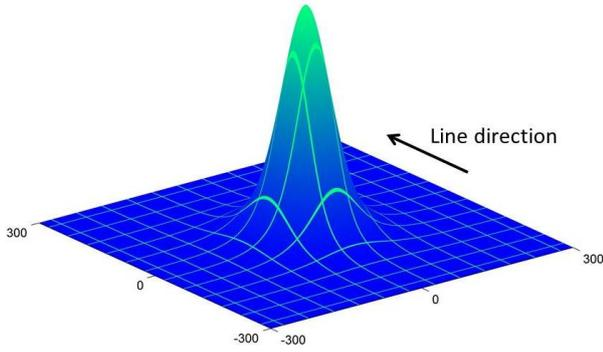
**Figure 1.** Source-detector response for a slab detector at 60 m height above a vertical rectangular prism source centred at (0,0) with dimensions 50×50 m. The figure is 600 m wide in the x and y dimensions.
