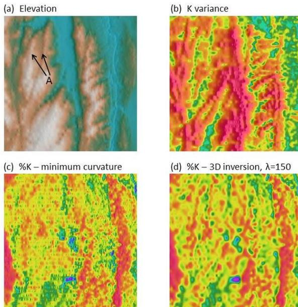
**Figure 3.** Pseudo-colour images from the SE Lachlan survey area: (a) digital elevation model, (b) K concentration variance, (c) K concentration (%) gridded using minimum curvature, and (d) K concentration gridded using 3D inversion. The images are centred on (149:04:39.99 E, 35:40:25.74 S) and are about 15 km wide. (Data courtesy of the Geological Survey of NSW)
