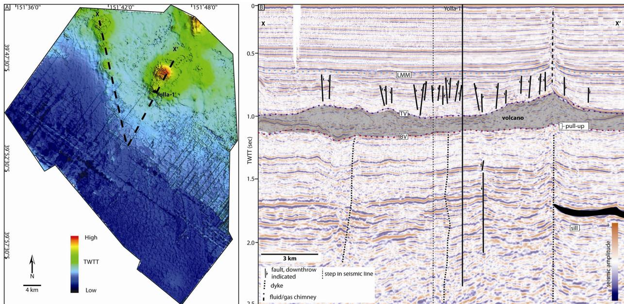
**Figure 1. Time map (A) and seismic cross section (B) in the Yolla survey showing the volcanoes. LMM= Lower Mid Miocene, TV=Top Volcanic, BV=Base Volcanic.**
