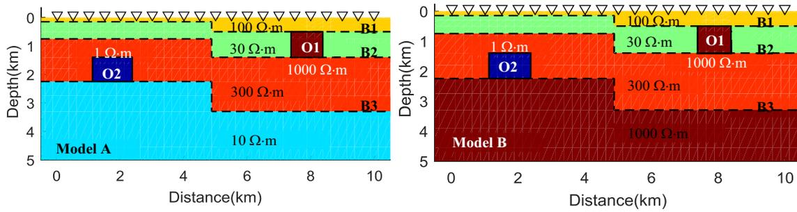
Figure 1. 2-D geo-electrical models, model A is the same as model B except the resistivity of the basement is changed. The three boundaries B1, B2 and B3 (dashed lines) divides the section in four layers. The two objects O1 and O2 are superimposed in the second and the third layer respectively. The triangles on the top profile mark the position of MT stations
