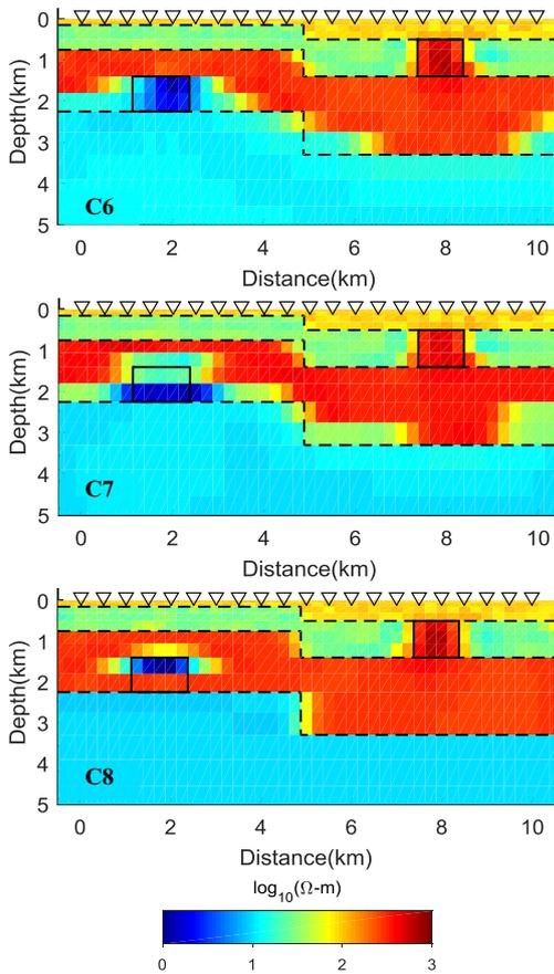
Figure 3c. Inversion results of model A using the information of two boundaries: B1 and B2 (C6); B1 and B3 (C7); and B2 and B3 (C8) and no the petrophysical information. Even with less boundary information at depth the reverred models are very good.
