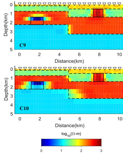
Figure 3d. Inversion results of model A using the information about the three boundaries and without (C9) and with (C10) the petrophysics. The inclusion of some boundary location information and that the earth is composed of discrete units allows very good recovery of the "true" model.
