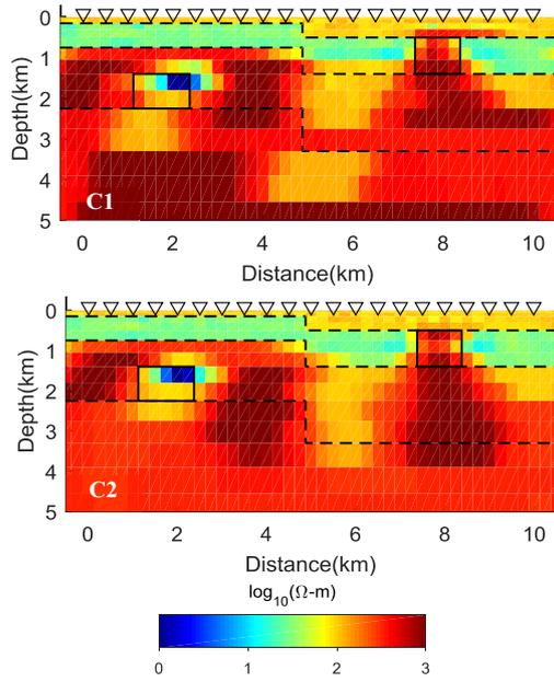
Figure 4a. Inversion results of model B without (C1) and with (C2) the prior petrophysics and no information about boundaries. The first, the second layers and the two objects are well defined, but the boundary between the basement and above layer is unrecovered because it is resistive media and the contrast of conductivity is small.
