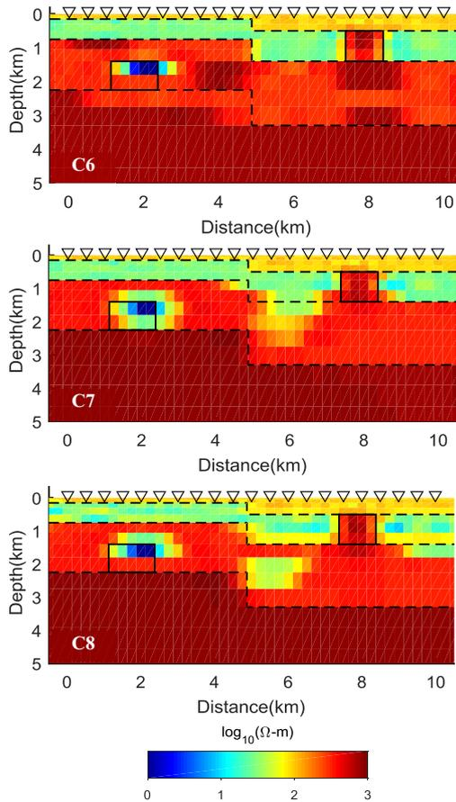
Figure 4c. The resulting inverted electrical resistivity distribution of model B using the information of two boundaries: B1 and B2 (C6); B1 and B3 (C7); and B2 and B3 (C8) and without the prior petrophysics. The inversion shows better result than the cases with only one boundary is added as the constraint.
