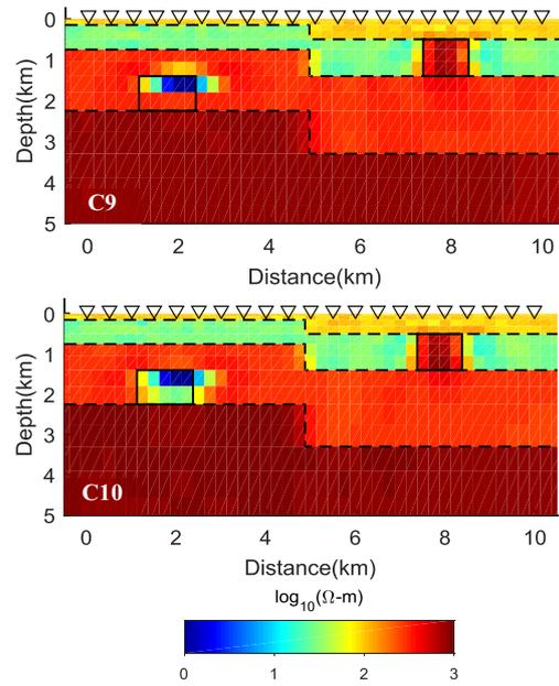
Figure 4d. Inversion results of model B using the information of the three boundaries and without (C9) and with (C10) the prior petrophysics. The inverted results are almost 'true' model. It is worth noting that the information of the two objects is initially unknown.
