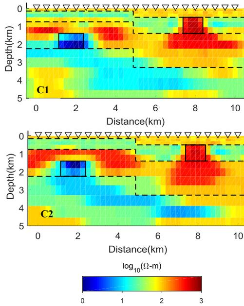
Figure 3a. Inversion results of model A without (C1) and with (C2) the prior petrophysics and no information about boundaries. Both are better than smooth inversions. Just the knowledge that the earth is made of discrete units assists inversion greatly.
