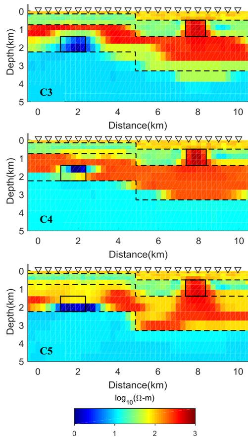
Figure 3b. Inversion results of model A using the information of one boundary: B1 (C3); B2 (C4); and B3 (C5) and no the petrophysical information. In this case the inclusion of the uppermost boundary information makes the greatest difference.
