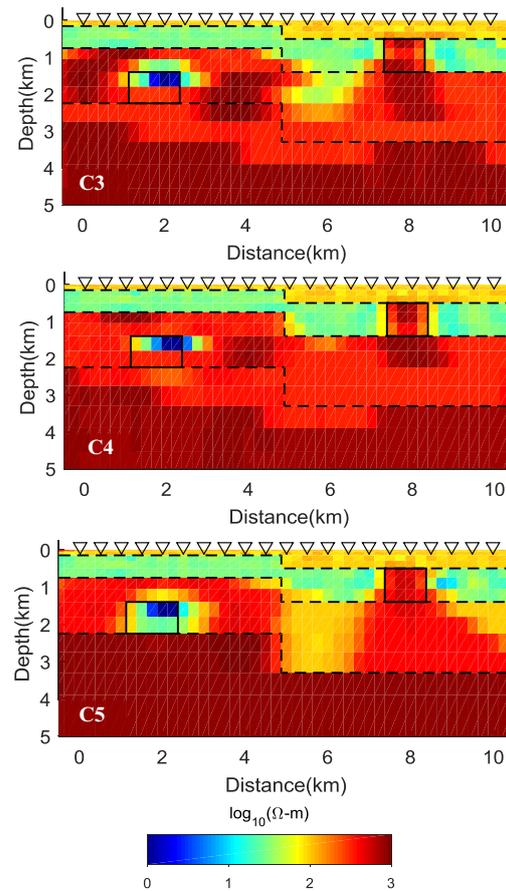
Figure 4b. Inversion results of model B using the information of one boundary: B1 (C3); B2 (C4); and B3 (C5) and without the prior petrophysics. The inclusion of one boundary information makes a significant improvement in comparison with the cases without boundary information.
