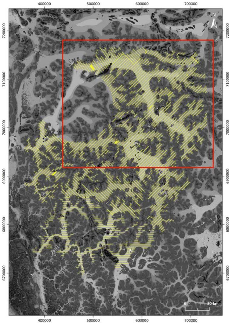
**Figure 4: Final flight line orientation map for the Murchison AEM survey.** Survey lines are overlain on a MrVBF map derived from the SRTM 1 sec DEM. The Flight lines were orientated, where possible, perpendicular to the expected orientation of the buried palaeovalleys that were expected to occupy the low, flat parts (pale grey areas) of the contemporary landscape. Total number of line kms acquired over the area was 14 069, comprising 1096 lines.
