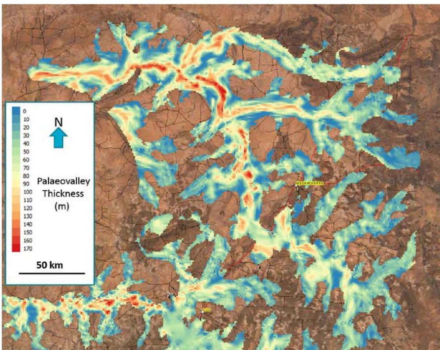
**Figure 5: Palaeovalley thickness map for northern part of Murchison survey area** derived from a 1D LEI of SkyTEM data acquired across the region. The thicker sequences of valley fill are mapped in reds and yellows.
