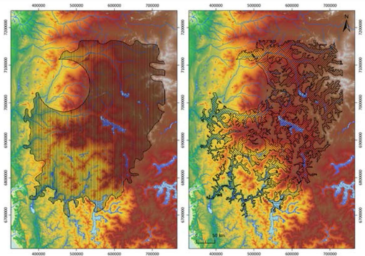
Figure 3: Comparison between a “conventional style” survey acquisition plan (left panel) versus a targeted survey approach (right panel) as was adopted in the Murchison region. The maps show survey extent and proposed AEM survey lines at 4km line spacing draped on SRTM 1 sec DEM. The total area covered by the bounding line in left panel is 106 283 km<sup>2</sup>. The actual area flown (right panel) was 51 284 km<sup>2</sup>.
