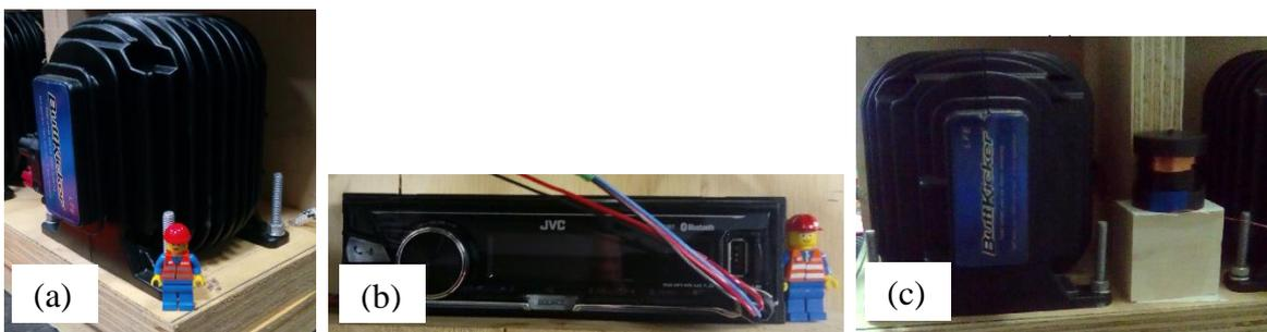
**Figure 3. Photos of (a) the buttkicker actuator and (b) the stereo with the auxiliary cable connected to a laptop.**
