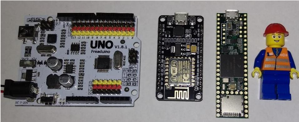
**Figure 6. Photos of different Arduino boards (from left): Freeduino (\$30), NodeMcu (with integrated WiFi, \$10), and Teensy 3.6 (with integrated micro-SD card, \$40).**
