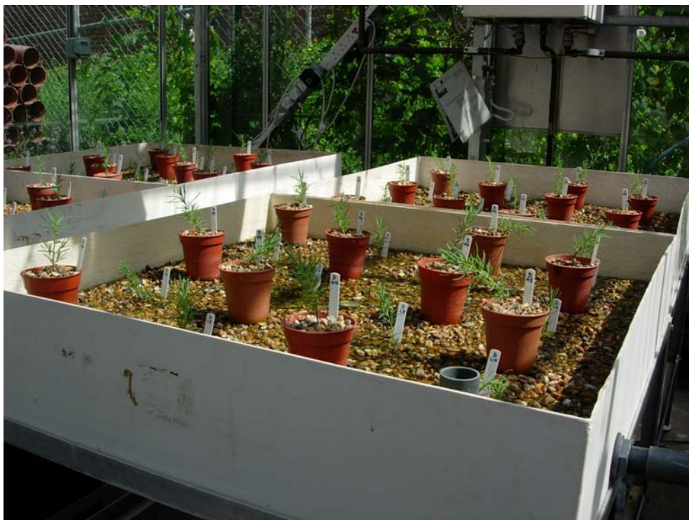
Fig. S2. (a) Diagrammatic representation of the simulated tidal flow tank system for creating fluctuating waterlogged conditions in pots of Suaeda maritima . Seawater was pumped from the reservoir into the gravel-filled tank to a maximum depth of 18 cm after which the seawater returned down the overflow pipe back to the reservoir tank. A minimum seawater height of 9 cm was maintained when the pump was off and seawater drained down to the height of the central pipe at the level of the top of the gravel. (b) Photograph showing Suaeda maritima plants growing in pots on top of or sunk into the gravel in the tanks of the glasshouse tidal flow tank system.
