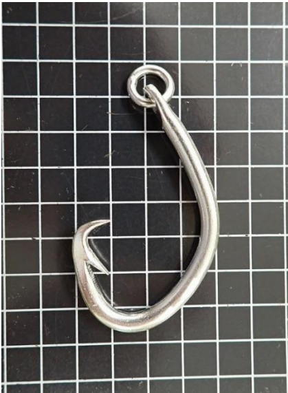
Fig. S1. Figure of hooks used in the experiment, including a 1-cm 2 background. Images for Hisamatsu Tankichi, Uruwa hook BKN 3.8 sun; Doitomi, Tuna circle hook SS-170 #4; Komatsu Keisaku, Circle hook type North America 5.2 sun; and Pacific Fishing Tackle MFG., CO. Circle hook 18/0 were copied from Yokota et al. (2006).
