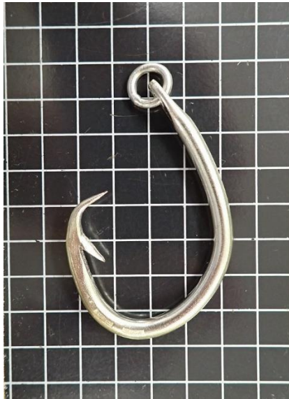
Fig. S1. Figure of hooks used in the experiment, including a 1-cm 2 background. Images for Hisamatsu Tankichi, Uruwa hook BKN 3.8 sun; Doitomi, Tuna circle hook SS-170 #4; Komatsu Keisaku, Circle hook type North America 5.2 sun; and Pacific Fishing Tackle MFG., CO. Circle hook 18/0 were copied from Yokota et al. (2006).
