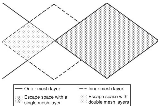
**Fig. 6.** Space for juveniles to escape from fish fences with single and double layers of mesh.
