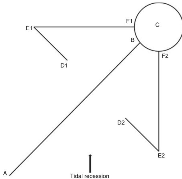
**Fig. 1.** Typical design of a fish fence. The dimensions vary, but the fish fences always follow this simple design. Spine length is calculated as the distance between A and B. Wing length is the combined length of  $D1 \rightarrow E1 \rightarrow F1 + D2 \rightarrow E2 \rightarrow F2$ . Aperture is the distance between D1 and D2. Mesh measurements were taken at collection point C only.
