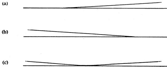
Fig. 4.—Idealized appearance of range duplications on fixed frequency records.
