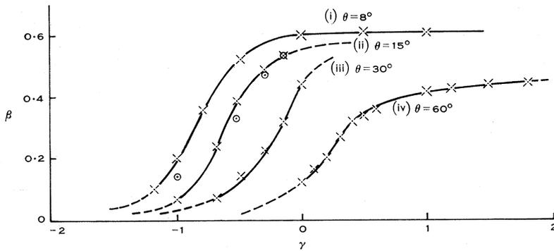
Fig. 4.—The graphs of  $\beta$  against  $\gamma$ , where  $\gamma = \log_{10} v/l$  for  $\varphi = 0^\circ$  and (i)  $\theta = 8^\circ$ , (ii)  $\theta = 15^\circ$ , (iii)  $\theta = 30^\circ$ , (iv)  $\theta = 60^\circ$ . In these cases,  $\alpha = 0.1$  and  $\kappa_0/l = 10^{-5}$ . The points plotted thus,  $\odot$ , are values of  $\beta$  calculated for  $\alpha = 0.2$ ,  $\theta = 15^\circ$ , and  $\kappa_0/l = 10^{-5}$ .
