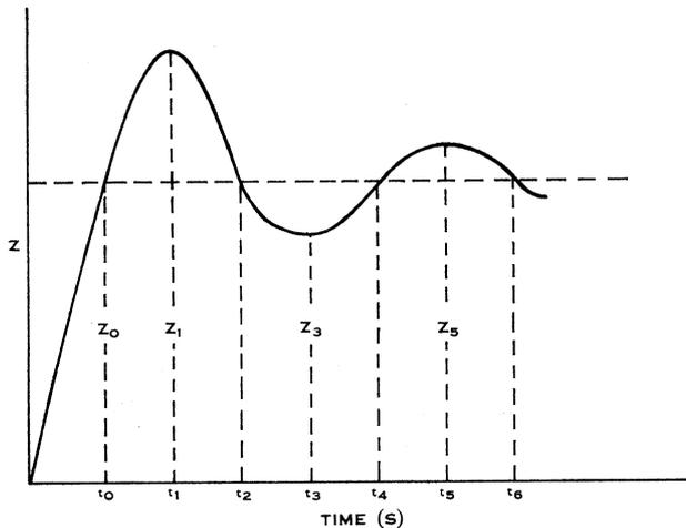
Fig. 1.—Oscillatory transients,  $Z = \text{temperature}$ .
